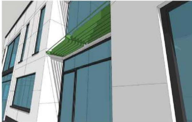
Brise Soleil over entrance
